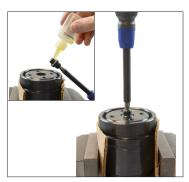
7. Apply oil to the piping adapter, then install into the bottom center port using a hex key. Use a torque wrench to tighten adapter to appropriate value listed in the table below.
