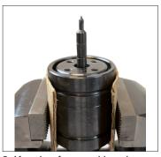
3. Keeping face and hands clear of the port, use either the 90.320.8 Port Servicing Tool or the 90.360.4 Valve Bleed Tool to depress the 90.260 Compact Valve. Cover the port with a cloth to absorb discharge.
