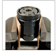
6. Position the gas spring upside down in a vise to secure. Be sure to wrap the cylinder body in cardboard to protect from damage.
