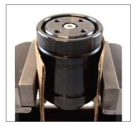
1. To exhaust pressure, secure the gas spring upside down in a vise body. Be sure to wrap the cylinder in cardboard to protect from damage.
