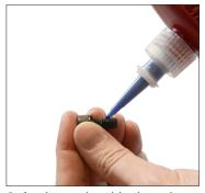
9. Apply serviceable thread locker to the bottom three threads of the cap screws with lockwashers.
