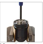
2. Remove the port plug located on the bottom of the spring with a 90.320.8 Port Servicing Tool.
