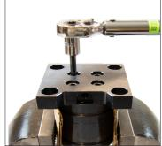
10. Fasten the mount by installing the cap screws with lock washers. Alternate tightening each screw 1/4 turn at a time (like a tire) to avoid pinching the adapter o-ring. With a torque wrench tighten the screws to the appropriate value listed in the table.
