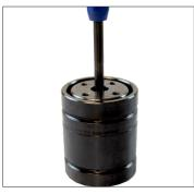
5. Remove the 90.260 Compact Valve using a 90.320.8 Port Servicing Tool.
