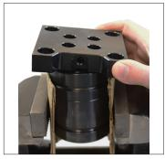
8. Align the B50 mount so that the piping adapter matches the hole in the mount, and cap screw holes align.
