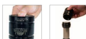
1. Choose the appropriate repair kit. The repair kit number needed is laser marked on the back of the Tube Assembly. Lightly polish out any scratches at the mouth of the Tube Assembly to avoid damaging seals during the reassembly process. If damage to the Tube Assembly is severe it must be replaced. Wash, clean and dry the inside thoroughly.
