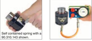
1S. Thread the Quick Disconnect Filler Valve, (90.310.143 or 90.310.111), into the port of the gas spring. Connect the female end of the charging assembly to the charging nipple. The DADCO Pressure Analyzer, (90.315.5), can also be used for charging, discharging and gauging pressure in self contained gas springs.
