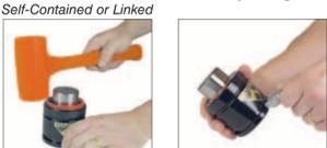
9. Install the new Dust Cover, (90.246.U.x). Tap with a soft mallet until the top of the Dust Cover rests flush with the top of the can. The rod wiper should be visible.
