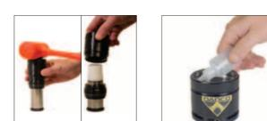
2. For applicable sizes, thread Assembly Cone (90.331.x) from Cartridge Starter Kit (90.335.x) onto rod. Be careful not to force the cartridge at an angle as the seal could become damaged.
