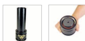
1. Stand the gas spring upright. Place a removal sleeve, (90.340.x), longer than the stroke over the rod. Tap the sleeve until the Dust Cover, (90.246.U.x), is loosened. Remove the Dust Cover and discard.
