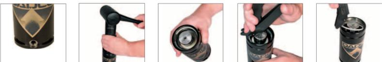
1. Stand the gas spring upright. Place a removal sleeve, (90.340.x), longer than the stroke over the rod. Tap the sleeve until the dust cover, (90.246.U.x), is loosened. Remove the Dust Cover and discard.
