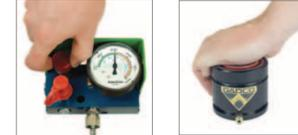
1L. Exhaust nitrogen gas by opening the bleed valve on the control panel.
