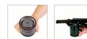
3A. While holding the cartridge, vertically lap the Assembly Cap to drive the cartridge down the rod. Be careful not to force the cartridge at an angle as the seal could become damaged.
