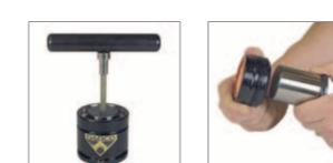
2. Once the cartridge and rod are removed from the Tube Assembly slide the cartridge off the rod and discard. Retain the rod for inspection and reuse.
