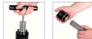
1. To remove the Rod and Cartridge Assembly thread a T-Handle, (90.320.2 or 90.320.10), into the rod end. Pull the entire assembly out of the tube. The spring body can be held in a vise (with soft jaws) while pulling out the assembly.
