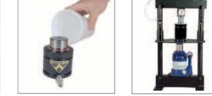
3. Open the main valve on the nitrogen tank. Set the desired charging pressure on the regulator. Do not exceed the maximum charging pressure of 150 bar (2175 psi).
