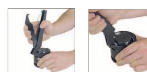
1. To remove the Rod and Cartridge Assembly thread a T-Handle, (90.320.1, 90.320.2 or 90.320.10), into the rod end. Pull the entire assembly out of the tube. The spring body can be held in a vise (with soft jaws) while pulling out the assembly.
