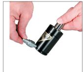
1. To increase the spring pressure, thread the Quick Disconnect Filler Valve, (90.310.143), into the port, set the regulator to the desired pressure and fill. The 90.315.5 may also be used to adjust pressure.
