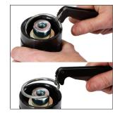
4. Once the hooked end of the tool is firmly seated below the c-ring, begin pushing it toward the outside of the gas spring tube. The handles will close naturally, and the c-ring will be extracted as you complete this motion. For a detailed explanation of c-ring removal see bulletin #B13113C.
