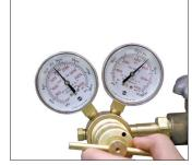
3. Set the desired charging pressure on the regulator. DADCO recommends charging the spring to the maximum charging pressure of 150 bar (2175 psi).
