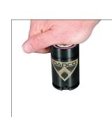
4. After all of the gas pressure is exhausted, be sure that the piston rod will freely retract into the tube manually. If not, try depressing the valve again. If still unsuccessful stop and contact DADCO.
