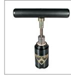
1. To remove the Rod and Cartridge Assembly thread a T-Handle, (90.320.M), into the rod end. Pull the entire assembly out of the tube. The spring body can be held in a vise (with soft jaws) while pulling out the assembly.
