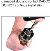
7. Thread the T-Handle, (90.320.M), into the end of the piston rod. Pull up on the T-Handle until the top of the cartridge is completely past the c-ring. The rod must seat the cartridge assembly fully before
