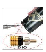
4A. Thread a new Compact Valve, (90.260), into the port until it fits snugly on the seat. Avoid over torquing the valve.
