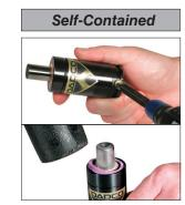
8. Install the new Dust Cover, (90.246.x.x). Tap with a soft mallet until the top of the Dust Cover rests flush with the top of the Tube Assembly. The rod wiper should be visible. 9. Thread the Port Plug
