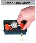
1. Exhaust nitrogen gas by opening the bleed valve on the control panel.
