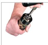
charging. The cartridge should be flush with the end of the cylinder. Make sure the rod is extended to its proper stroke length. (Depress the needle valve to facilitate full rod extension.)
