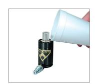
7. Check for leaks at the top of the tube around the rod and at the base around the valve
