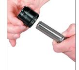
2. Once the cartridge and rod are removed from the Tube Assembly slide the cartridge off the rod and discard. Retain the rod for inspection and reuse.
