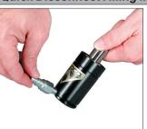
1. Thread the M6 end of the Quick Disconnect Filler Valve. (90.310.143), into the port of the gas spring. Connect the female end of the charging assembly to the charging nipple. The DADCO Pressure Analyzer. (90.315.5). can also be used for charging discharging and gauging pressure.
