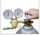
2. Open the main valve on the nitrogen tank.
