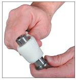
1. Lightly polish the rod surface with an emery cloth (600 grit). Inspect the finish of the rod for any scratches or gouges. If the rod is damaged it must be
