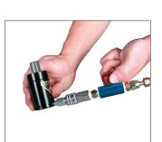
5. Turn the Shut-off Valve until it aligns with the CLOSE AND VENTED position located on the lower black knob. If using the Standard Charging Assembly (90.310.040), the small amount of nitrogen trapped between the shutoff valve and filler valve will escape as you disconnect from the spring.
