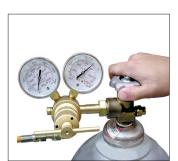
6. After all the springs in the system have been charged to the desired pressure, CLOSE THE HOSE SHUT-OFF VALVE AND TANK SHUT-OFF VALVE.
