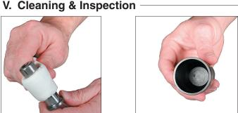
2. Inspect the Tube Assembly for any damage, especially around the mouth of the Tube Assembly. Lightly polish out any scratches at the mouth of the Tube Assembly to avoid damaging seals during the reassembly process. If damage to the Tube Assembly is severe it must be replaced. Wash, clean and dry the inside thoroughly.
