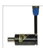
3. Keeping face and hands clear of the port, use the Valve Bleed Tool, (90.360.4), or Port Servicing Tool. (90.320.8). to depress the valve stem (90.250) or (90.260). Cover the port with a cloth to absorb discharge.
