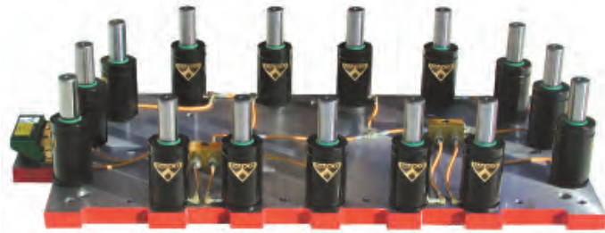
DADCO SMS® with fifteen 90.9.01500 cylinders linked using 90.700 (Y-700) hose with permanent hose adapters. This system employs two distribution blocks to simplify piping to a mini control panel that is used to drain, fill and monitor the pressure from outside the die. Contact DADCO for more information on linked operations.
